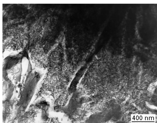
Figure 6 A bright field image featuring crystals of CAH 10 embedded in alumina gel.
